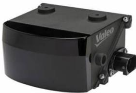
Valeo SCALA 2 is new generation of Valeo SCALA, which is the first automotive grade laser scanner on the market, making its debut in 2017 with a German premium brand and the 2018 PACE award winner. Valeo SCALA 2 offers 3 times wider vertical field of view from its previous model enabling for example lane marking detection. It works during day and night at both low and high speeds, scanning its environment for any kind of obstacles. Valeo SCALA
