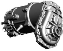
Valeo also makes the **48V Electric Rear Axle Drive Light**, full propulsion system based on 48V Gearbox Motor Generator, its debut in Japan. Having up to 19kW at peak and 12 kW in continuous, it is compatible with vehicles weighing up to 1,200 kg such as Kei-cars, heavy quadricycles (L7e) and Low-speed Electric Vehicle (LSEV). Its lightweight (less than 25 kg) and compact size allow an easy integration.
