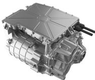
Regarding the high-power solutions, Valeo Siemens eAutomotive has developed **High Power eDrive 100kW** combined with an inverter and reducer. It has a common liquid cooling system for Motor, Inverter & Transmission. It Integrated eDrive platform perfectly suited for vehicle platforms with a broad power range and a variety of drivetrain configurations.
